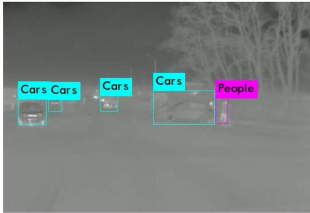
The example of traffic obstacles detection algorithm operation based on LWIR stereo camera data processing
